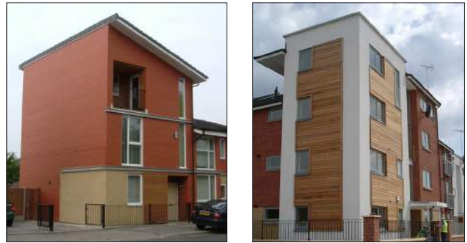
Fig 5.18: Left: the blank elevation has a deadening effect on the street scene. Right: building designed to positively address the corner.
