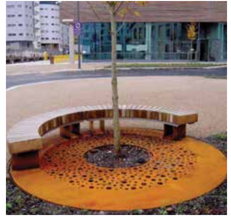
Corten tree grille and timber bench
